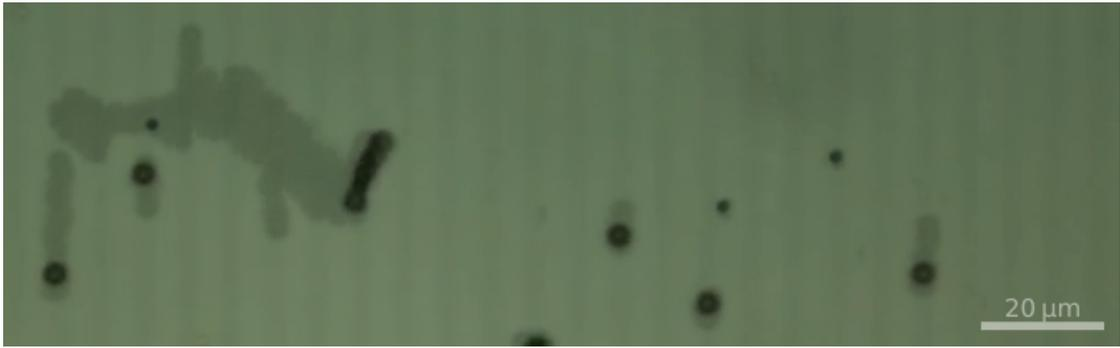
**Figure 15:** Typical experimental result for the walking motion. The figure consists of the overlaid frames in the first 5 s of Video 4 (accessible via the QR code). In this time, the low-frequency control loop from Figure 12 is driven five times while the low-frequency field is fixed pointing upwards. As predicted, single particles don't move forward and the biped moves to the right. More details are visible in the video and in Figure 16.
