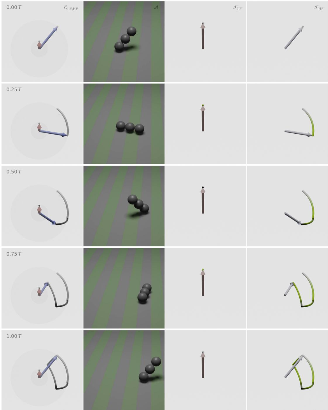
**Figure 6:** Brownian dynamics simulation results of a biped walking due to direction modulation of the high-frequency field amplitude  $\hat{\mathbf{H}}_{\text{HF}}$ . The snapshots are taken from Video 2 (accessible via the QR code) in intervals of  $0.25T$ , where  $T = 20$  s is the period of the adiabatic modulation of the amplitude (*not* the period of the high-frequency oscillation). The columns show the same spaces as in Figure 5.
