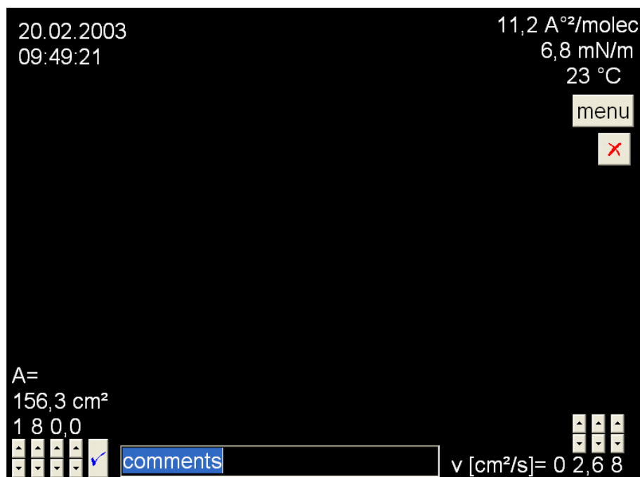
Figure A.11.1: Screenshot of the film balance control software. The computer image and fluorescence image from the SIT camera (positioned in the center) are overlaid by a Genlock adapter. Upper left corner: date and time. Upper right corner: area per molecule, surface pressure, temperature. Lower left corner: actual area and target area. Lower right corner: barrier velocity.
