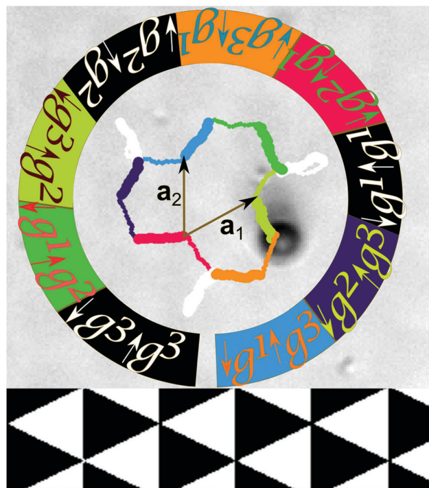
Fig. 19 Experimental trajectory of a paramagnetic colloidal particle on top of a S_6 pattern caused by a modulation poly-loop in \mathcal{C} consisting of a sequence of all fundamental modulation loops. The fundamental loops are colored according to the loops in the phase diagram in Fig. 14. South traveling segments are marked as thick lines. North traveling segments are marked as thin lines. A video clip of the motion of the paramagnetic colloidal particle is provided in ref. 45.
