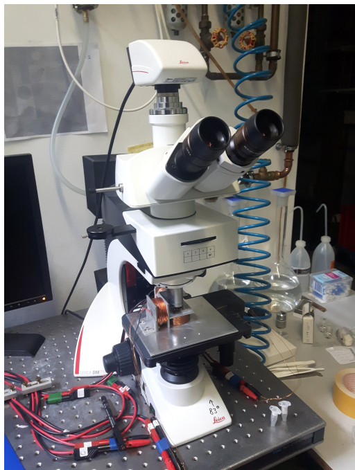
Figure 3.4: Image of the microscope used with coils for external magnetic field creation.
